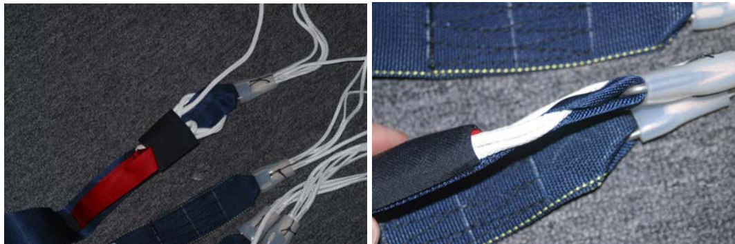
Improper way to set excess brake line on reserve risers
