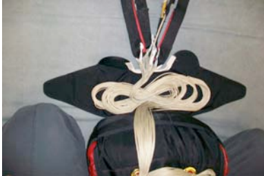
Fig. 9 – Stowed lines. Ensure that stowed lines do not exceed the width of the bag.
