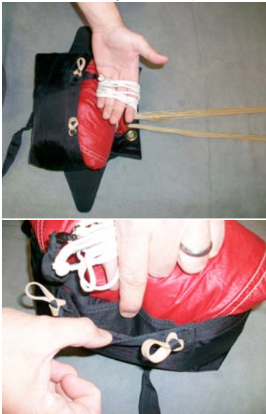
Fig. 3 - RDS line coiled, and placed in pocket (if used, ignore if not on canopy)
